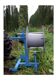
Fix the wire ends from a wire frame to the winding drum. However, first guide the gathered ends through the wire guide before inserting them through the slot on the winding drum or fixing them to the tension release device.
